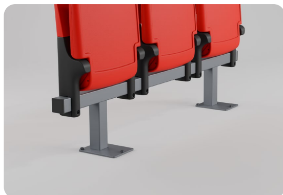
Seat mounted on a steel beam , using clamped or welded brackets , with an adjustable connection between the beam and the legs.
