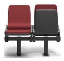
Folding seat with advanced controlled-return technology, ideal for sports facilities and multipurpose venues. Composed of upholstered cushions combined with polypropylene shells, it ensures exceptional performance and durability. Its automatic folding system for both seat and backrest provides great compactness when folded, optimizing space. Dimensions are 460mm width, 165 depth and 870 height.
